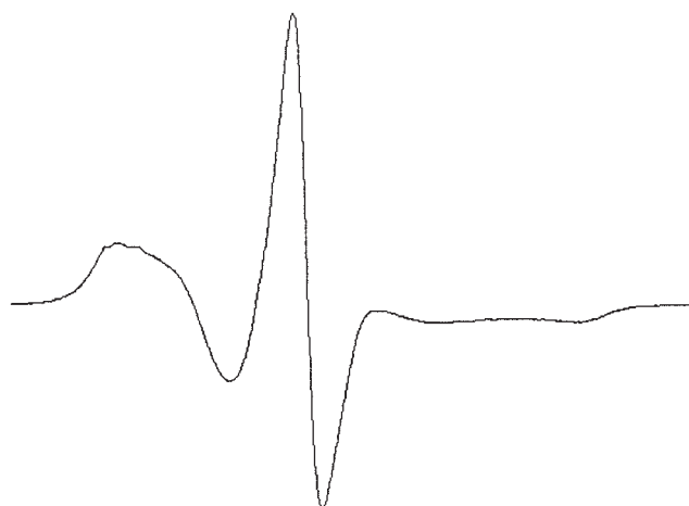
Figure 3 ESR spectrum of solid spin-labeled system.
